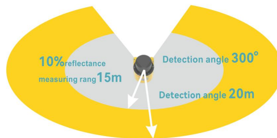
Figure 3.1 Measuring Coordinate System/Scan Range/Range
